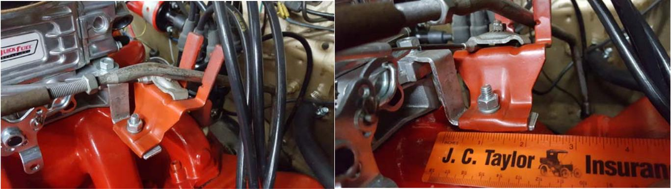
I then cut the original kickdown in the vertical section and welded in a ~5" section in to extend it.
