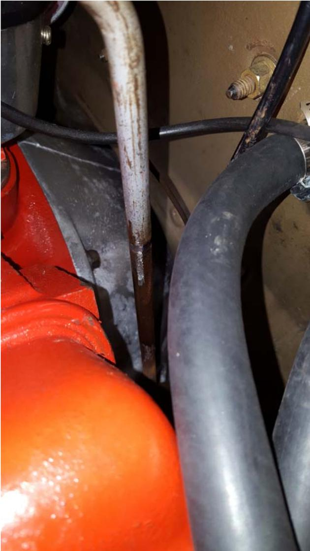
Next I found a steel sleeve and extended the original throttle return spring stand up ~2".
