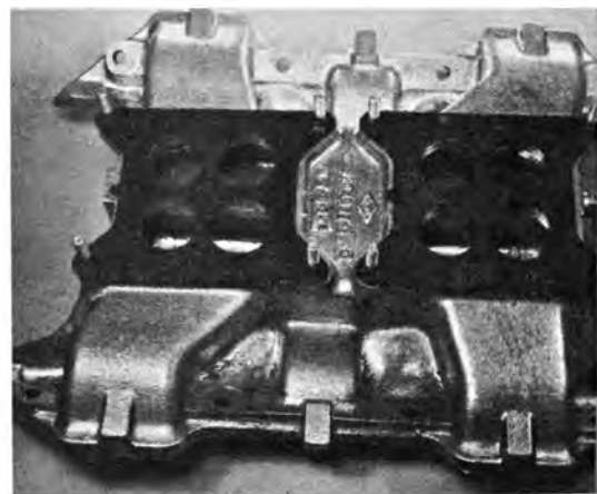
Dividing wall between manifold logs is visible. Some exhaust heat is supplied through the crossover, but it may be blocked-off quite simply.
