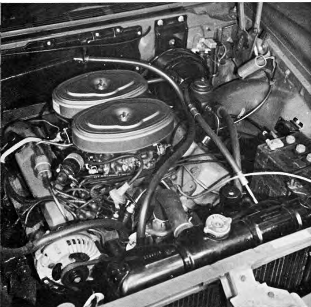
300H in its quickest street trim produces 380 horsepower from 413 cu. in. when fitted with this dual-quad carb manifold.
