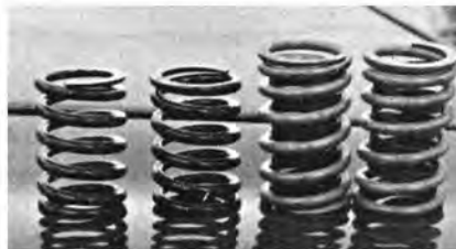
Stiffer valve springs with flat wound dampers help return big valves of 405 hp option.
